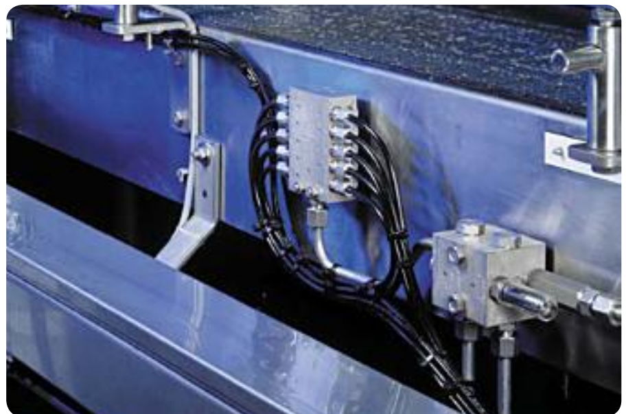
SSV and VSKH2-KR lubricant metering dividers at a conveyor belt (Beverage industry)
