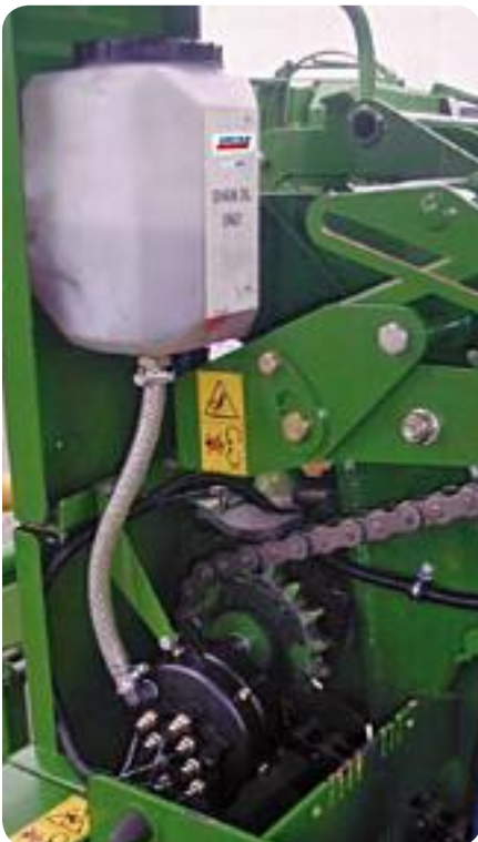
Agricultural machine (baler) with MOS/MOP 212 lubrication system
