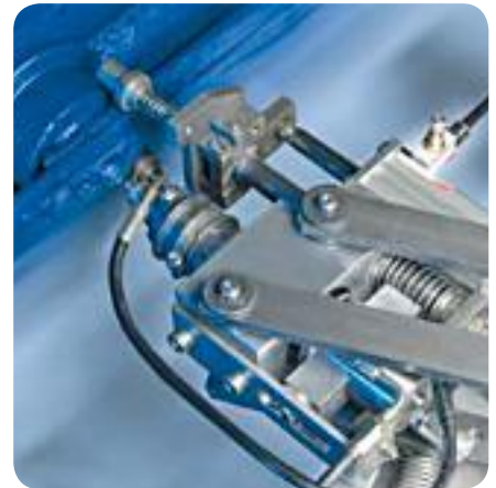
SSV and VSKH2-KR lubricant metering dividers at a conveyor belt (Beverage industry)
